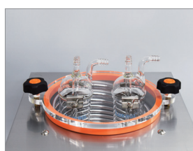
Glass Trap installed
